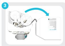
Be careful not to pull the wires attached to the cover. Rotate the cover and place it in front of the system.
