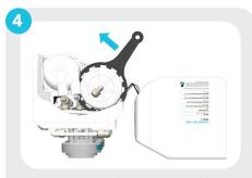
Disconnect tubing connected to membrane housing cap. Remove the caps using the included wrench, turning counterclockwise.
