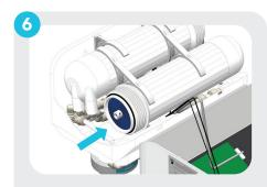
Make sure each membrane is fully seated in the housing.
