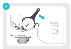
Reinstall both membrane housing caps and reconnect tubing.
