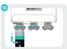
Slide the filter up into the head vertically and then rotate the filter to the right. Repeat for all 3 filters.
