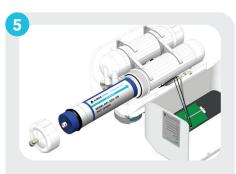
Lubricate each membrane's O-ring with food-grade silicone before inserting them into the housing.
