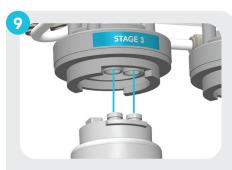
Match the filter label color to head label color and align the filter key.
