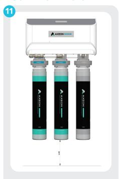
Mount RO System with a minimum 6 inches of clearance between the ground and bottom of the filter. Use mounting guide on page 23 of manual for hole alignment.
