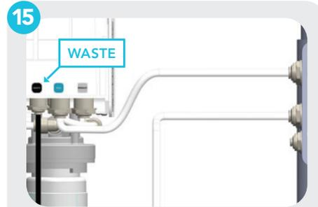
For wastewater, connect the 1/4" black tubing from the "WASTE" port on the RO system to the drain. Ensure it is unrestricted and has no back pressure.
